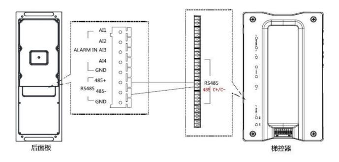
2. Go to the door station remote configuration->RS485 and select Bitrate: 19200 ->working mode->Stair control
